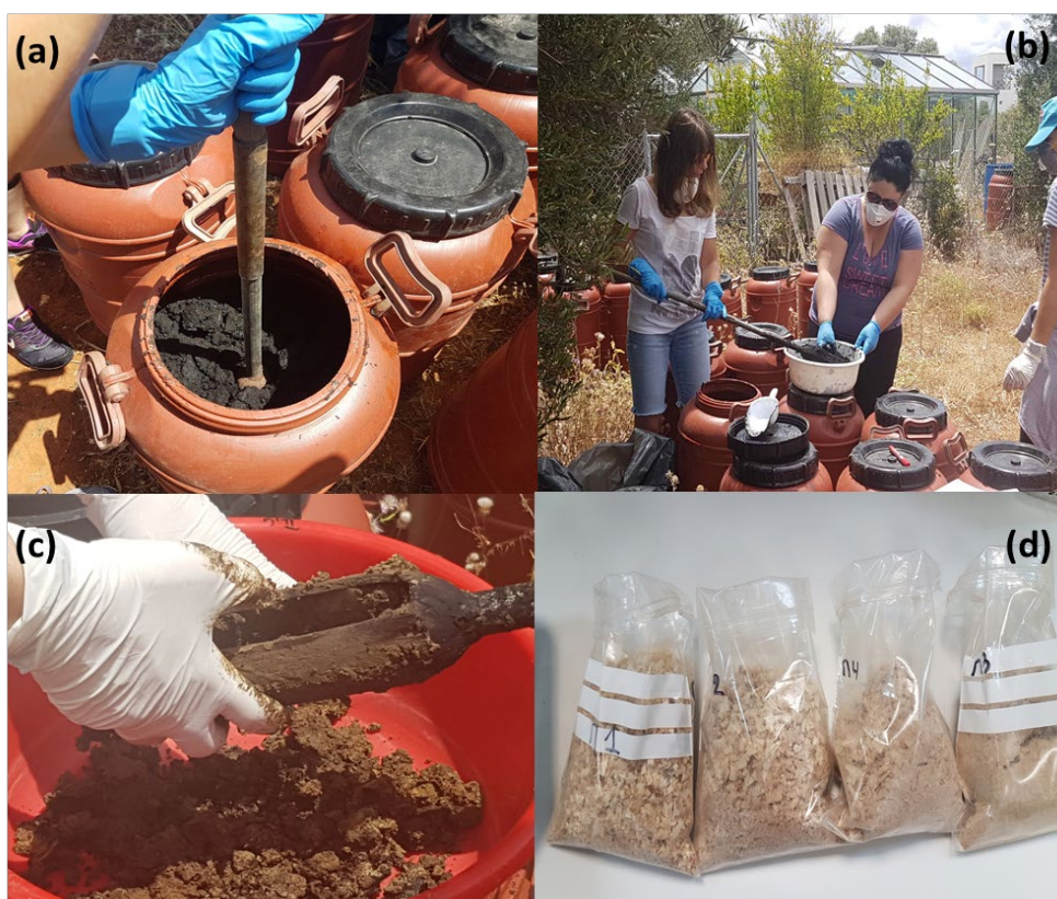
Figure 12. Sampling procedure of the feedstocks. a, b) Sewage sludge's sampling using auger, c) Olive Oil mill waste sampling using auger, d) Samples of sawdust
